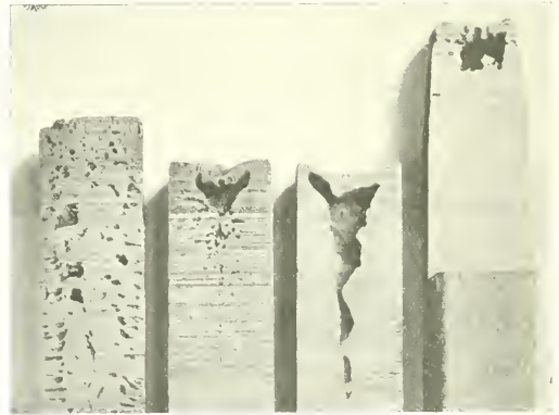
FIG. 2. Upper portion of four small ingots (1½ in. square) made to illustrate and test question of soundness and piping.
